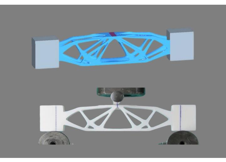
Optimization of solid and lattice structure three-point bending test: numerical and experimental results
